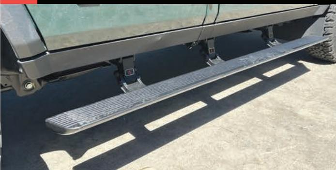
Electrically operated sidesteps extend and retract when the side doors are opened and closed. They are wired to an original switch in the Overhead Panel and can be switched off when driving offroad when greater ground clearance is required.
