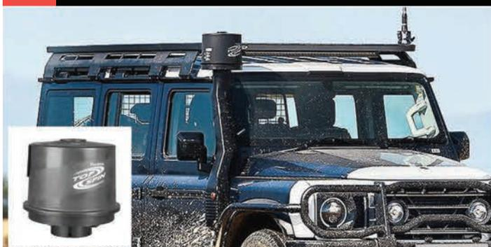
An additional filtering layer for the raised air intake. Provides the engine with cleaner airflow, keeping out dust and dirt by spinning the air as it enters the raised air intake, preventing contaminants from entering the intake duct.
