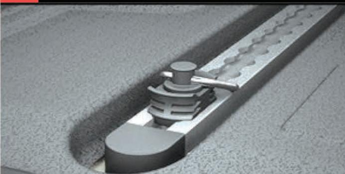
Utility rails fit into the floor of the rear compartments and allow for the secure fastening of loads and accessories. Quick release tie-down rings are required with this accessory.
