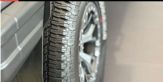
Wheel spacers move the road wheels towards the outer side of the body giving the vehicle a more aggressive and rugged appearance
