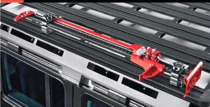
The secure way to carry a high-lift jack by fixing it to the roof rack.
