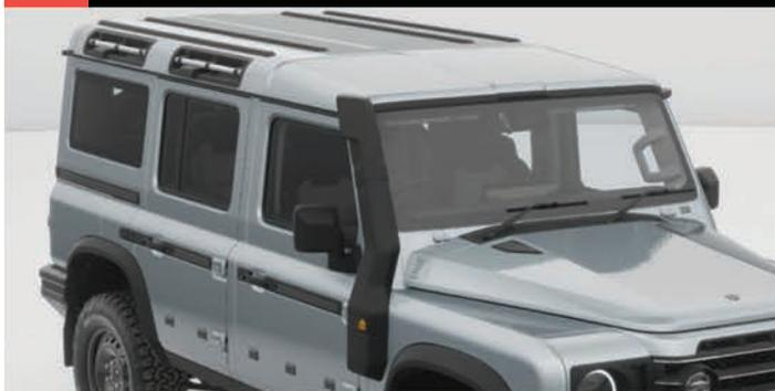
Raising the position of the engine air intake ensures the engine is fed with cleaner and cooler air in dusty environments.
