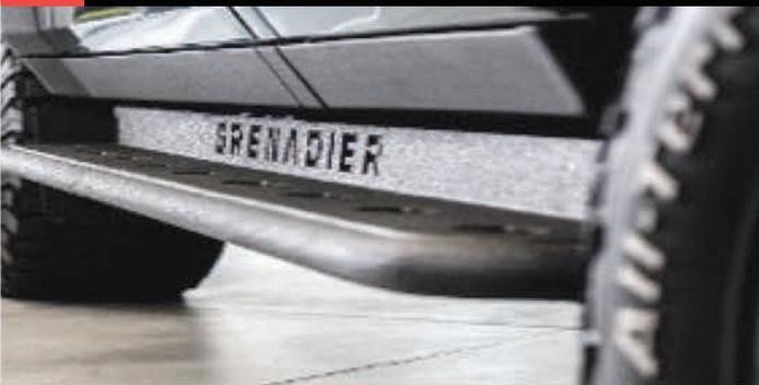
Sidesteps securely mounted to the chassis of the vehicle and make entry and exit much easier especially for children. Protected by a robust rubberised coating with "GRENADIER" laser cut into the step.
