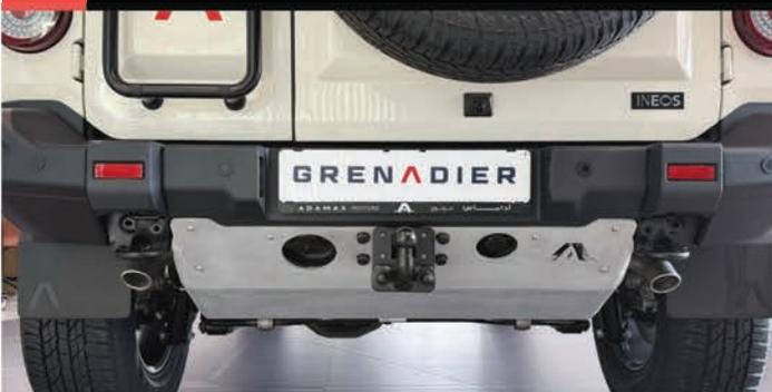
Heavy duty front and rear underbody protection with built in hitch receiver at the rear. Additional protection for the underbody area and improved ramp and departure angles when off- road.
