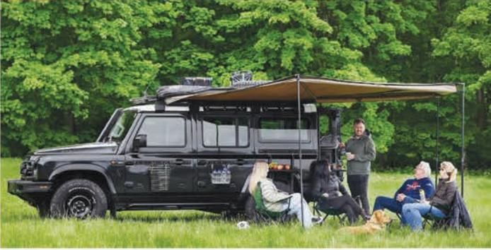
This awning is mounted on the side of the roof rack and deploys 270° to provide maximum shade and protection from the elements while camping. Note: Must be mounted to a Roof Rack or Ladder Rack
