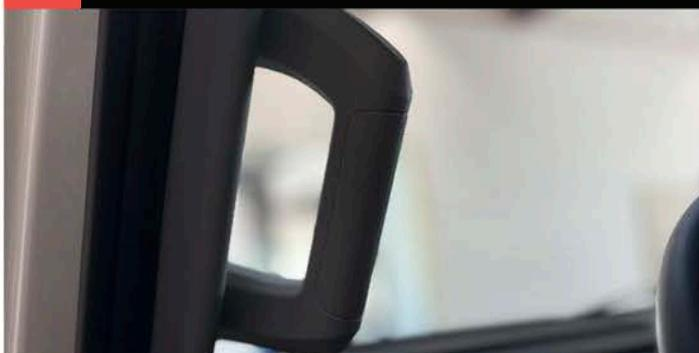
Additional handle mounts to the left A pillar and assist the driver when getting in and out of the vehicle. Matches and balances with the original handle mounted on the right a pillar.
