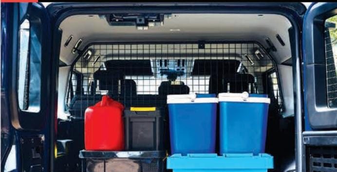
The cargo barrier helps increase safety inside your vehicle, by preventing loadspace cargo from entering the passenger's cabin and keeping pets and other contents safely away from driver and passengers.
