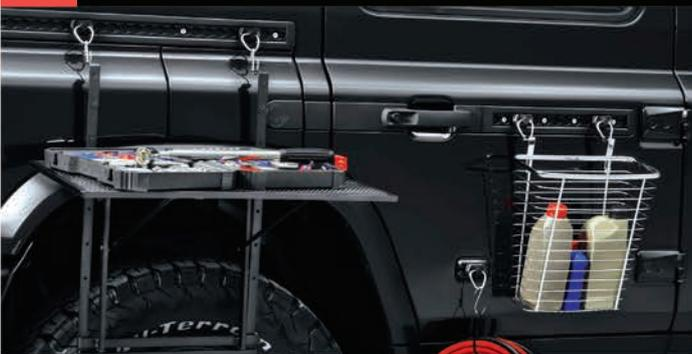
Quick release tie-down rings allow you to secure luggage or heavy loads to the utility rails on the sides and in the rear compartment floor of the vehicle.
