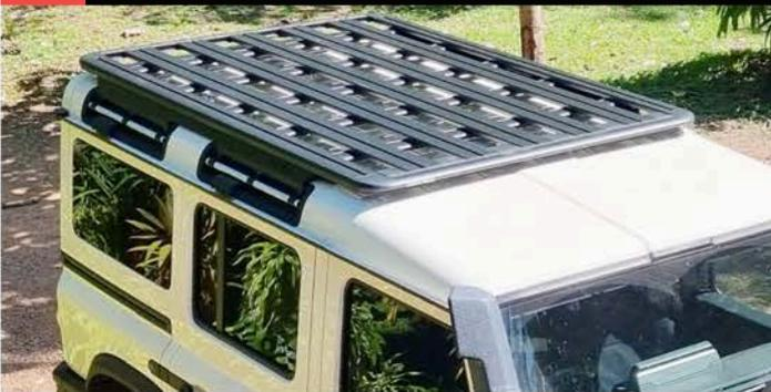
Shorter roof rack that's ideal for the Pick-Up, or to be used as a 3/4 length roof rack for the Station Wagon, this allows you to secure loads to the roof for extra carrying capacity. The shorter length also allows the Safari Windows to be opened.
