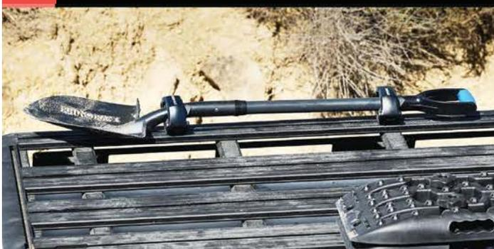
This bracket allows you to fix an axe or shovel in an easily accessible and secure place on the roof rack of your vehicle, to avoid using up cabin space.
