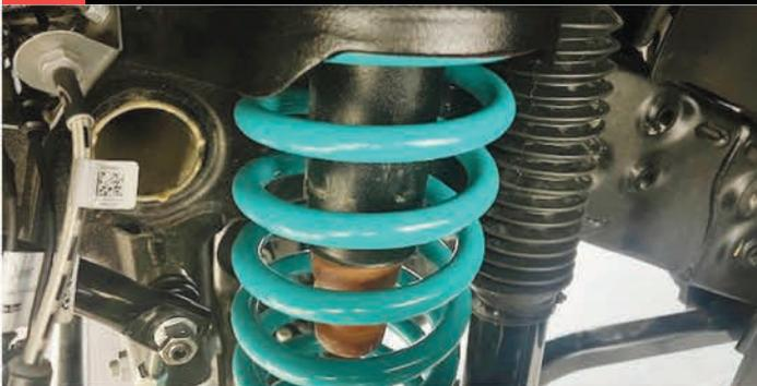
A spring lift kit raises the vehicle body and creates better ground clearance for use off road whilst giving a more muscular appearance. Also provides additional clearance when fitting larger wheel and tyre combinations.
